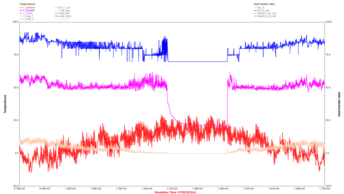
Figure 2: Red line = ambient temperature [°C], blue line = DH forward temperature [°C], pink line = DH return temperature [°C] and beige line = max. DH feed in capacity [MW].
